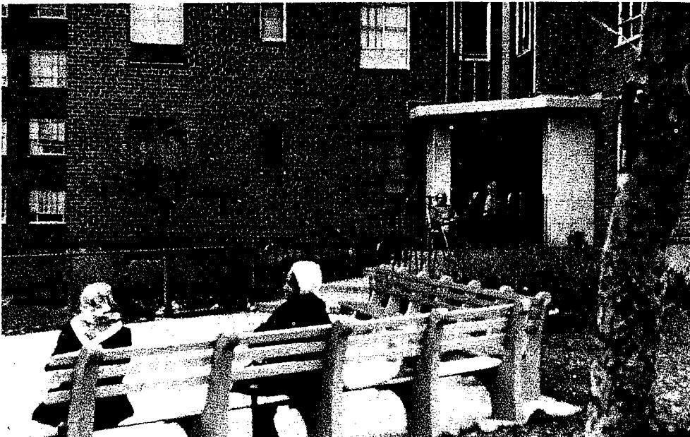
FIG. 52. Entry Buffer Area at Breukelen. View of entry to seven-story buildings—sitting and play area create semiprivate transitional zones which are further strengthened by sloped walk leading to entry doors. (Photo by author)
