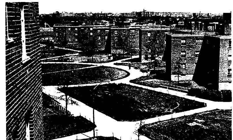
FIG. 33. View of the Interior Grounds at Breukelen. The interior grounds were designed to be open to public access from surrounding streets. They do not relate to particular buildings and house few defined activities. Residents view these interior areas as the most dangerous in the project. (Photo by author)
